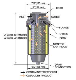
These housings installed with one Fuel-Gard® monitor
